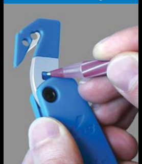
FILM CUTTER CHANGE Use ball point pen (above) to remove & replace film cutter unit.
